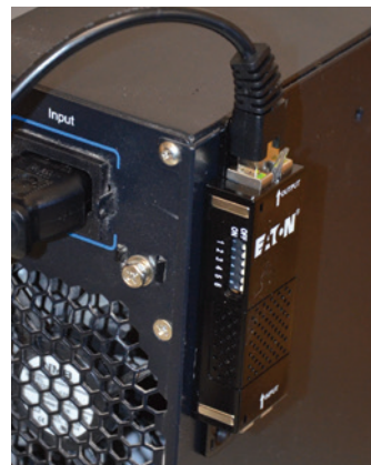
Eaton EMP Gen 2 installed
